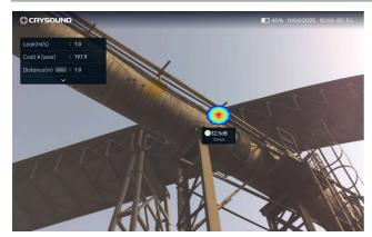
A coal chemical enterprise detected a gas leak in an overhead pipeline using the CRY8129-EX Acoustic Imaging Camera, which could not be identified by traditional methods.
