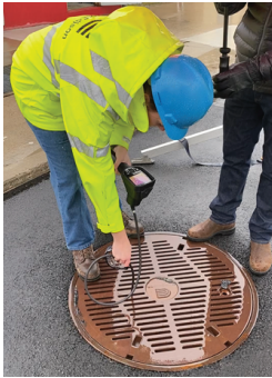
Figure 8.1 Inserting the probe into the test area.
