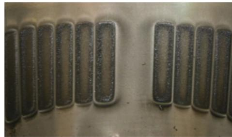
8.4 million particles captured and held by FilterMag. Most are small enough to pass through an engine oil filter.
