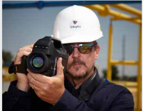
Optical gas imaging (OGI)
