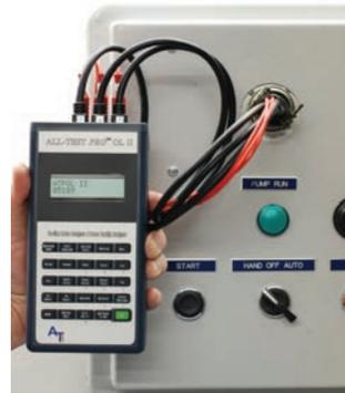
Enhance energized testing safety and improve testing productivity by installing the ALL-SAFE PRO® Connection Box. Bluetooth in ATPOL II™ allows for remote operation of the instrument.
