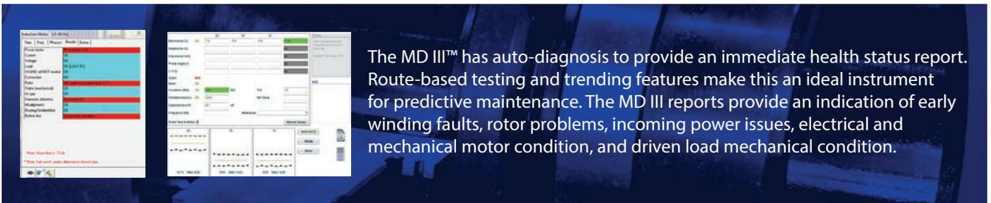
The MD III™ has auto-diagnosis to provide an immediate health status report. Route-based testing and trending features make this an ideal instrument for predictive maintenance. The MD III reports provide an indication of early winding faults, rotor problems, incoming power issues, electrical and mechanical motor condition, and driven load mechanical condition.
