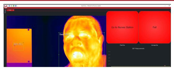
Do environmental conditions affect the temperature measurement reading from the camera? Yes. This is apparent when someone comes inside from cold weather conditions. The body and tear duct region is exposed to the cold, will read colder until the body normalizes and comes back up to temperature. This could take up to several minutes.
