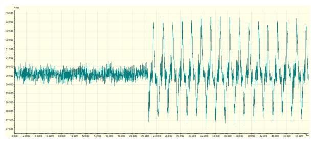
Figure 1. Results of initial test show the current waveform. There is evidence of strong load fluctuations (peak 6 amps at 20% of the total load). These fluctuations were determined to be caused by improper configuration of the VFD controller and it's PID.
