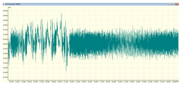
Figure 2. Energized motor testing with the ATPOL II™ shows the load performance is greatly improved after the VFD reconfiguration / PID correction.
