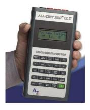
3. There are easy-to-use portable instruments, like the ALL-TEST PRO On-Line II™ energized motor testing instrument, that can help you check the health of your motors. The ATPOL II™ is an invaluable monitoring and diagnostic tool that can help you see what is really going on with your equipment. Make sure you have the proper tools to support your condition monitoring program.
