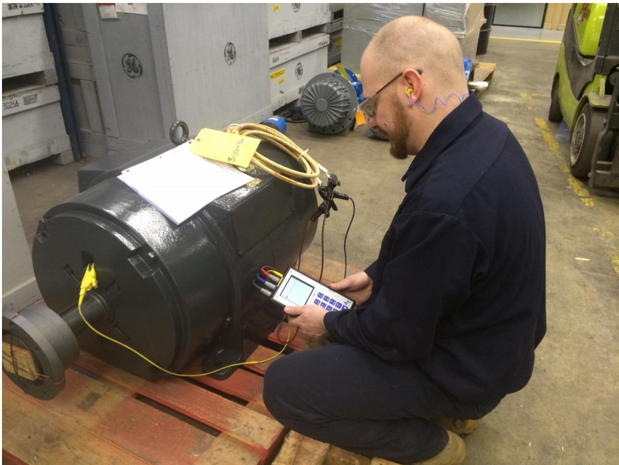
Koontz-Wagner Service Technician, Erik Lehman, utilizes the ALL-TEST PRO 5™ to perform initial inspection of a 50HP motor in the repair shop.
