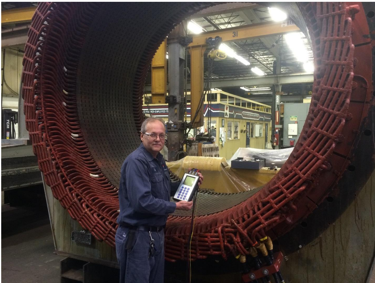
Ken Patterson, Head of the Predictive Maintenance Division at Koontz-Wagner, tests a 9000HP motor.
