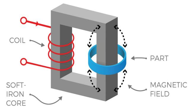
A low frequency induction field affects the complete part. The part heats equally.
