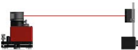
5-10 m between laser and detector
