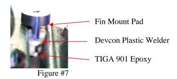
In tight locations the Devcon Plastic Welder could be applied with a syringe and taper tip to facilitate filling the voids between the walls of the motor fins and the fin mount pad. Once the Devcon Plastic Welder has cured (approximately 5-10 minutes), any bare metal may be painted, and the accelerometer mounted.
