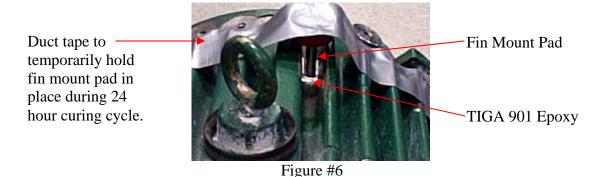
After the 24 hour curing cycle, the Devcon Plastic Welder can be added to fill the voids between the walls of the motor fins and the fin mount pad. This provides added strength to the mounting, but does not compromise the conductive bond that was established with the TIGA 901. This secondary epoxy fill will reduce mounting costs and provide side wall support for the fin mount pad as shown in Figure #7.
