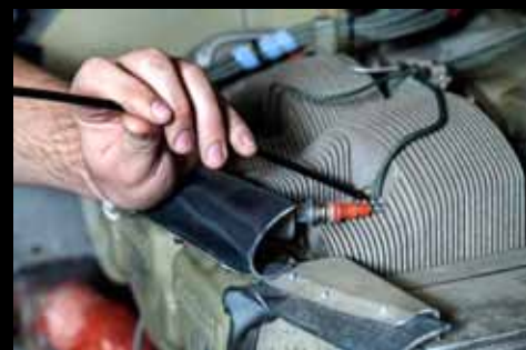
Inspecting cylinder in aircraft motor with VSA2-1M
