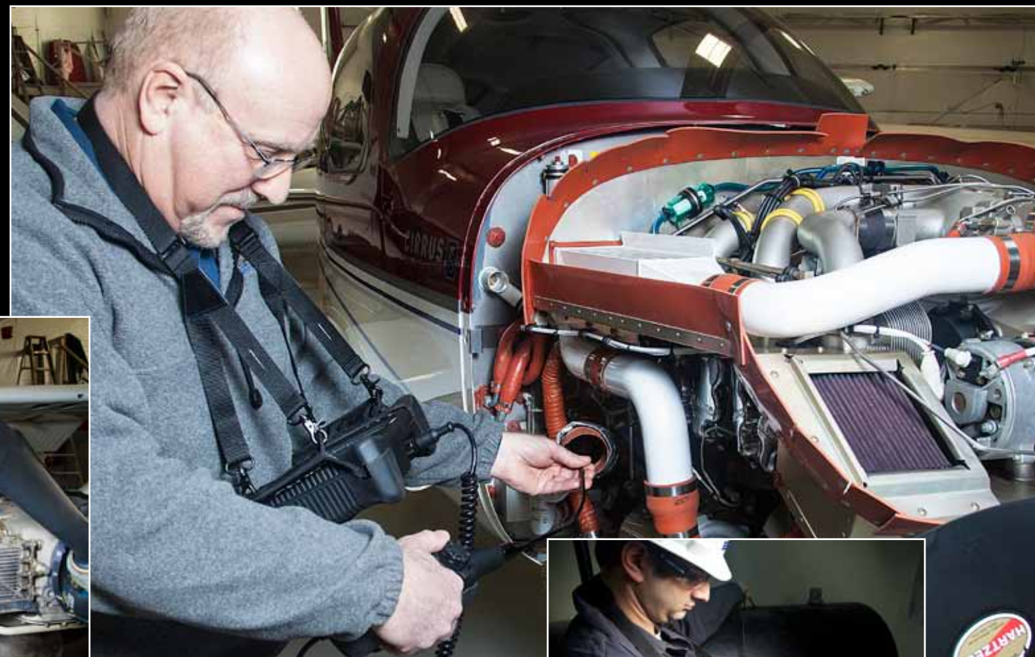
Checking aircraft engines and airframes for cracks, wear, defects and debris; inspecting oil tank for corrosion; Checking air duct for blockage.
