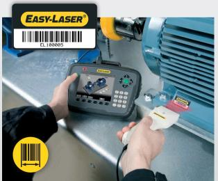
The barcode reader is used to enter the machine data before measurement is taken. After the first measurement is recorded, the adhesive barcode label is applied to the machine. Next time the machine is checked, the measurements, compensation values and tolerances can be read directly from the barcode. Simple and accurate!
