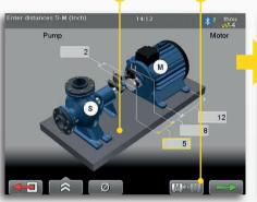
**1.** Enter the distances between measuring units and the machine feet. If you enter the coupling diameter you can also get the result as gap/sag.
