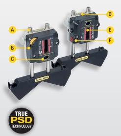
A. The rods have a height of 2.4"–7.0" [60–180 mm]. If necessary they can be extended "infinitely" with accessory rods. Made of stainless steel. B. Pre-mounted units/brackets C. Laser aperture D. Sturdy aluminum body E. PSD (1.2"/30 mm) F. On/Off button
