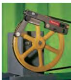
Tool is mounted magnetically against inside or outside face of pulley and the targets against the face of the opposite pulley. The laser-line projected from the end of the tool onto the targets allows the user to quickly ascertain and correct angular and offset misalignment between the pulleys. Only one person needed to perfectly align your drives!
