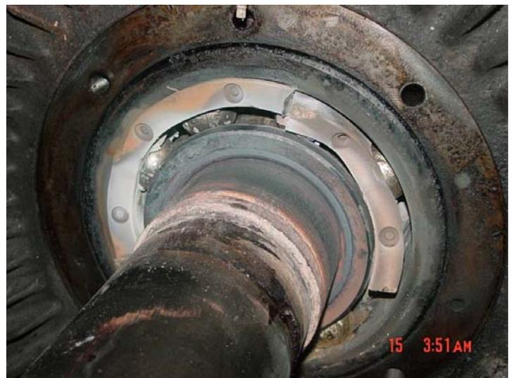
***Failed Motor Bearing
