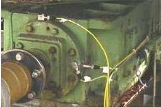
*Accelerometers on a Gear Box*
