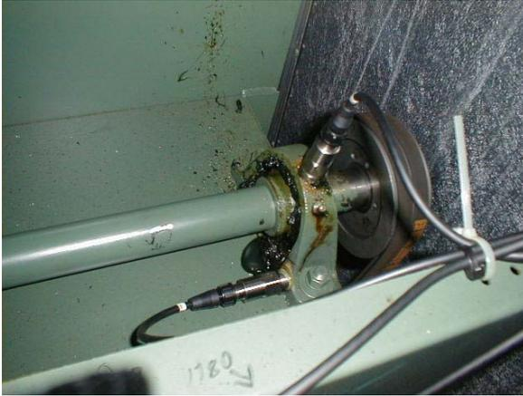
***Loop Power Sensors to Monitor Bearing Vibration***
